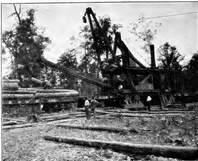
A STEAM SKIDDER IN USE BY THE SAWYER & AUSTIN LUMBER CO., PINE BLUFF, ARK.
